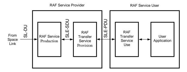
Figure 2-2: RAF Service Production and Provision
