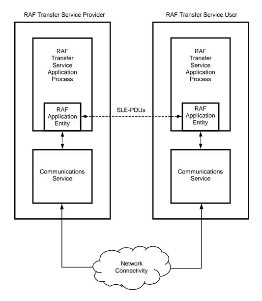
Figure 2-5: Communications Realization of RAF Service
